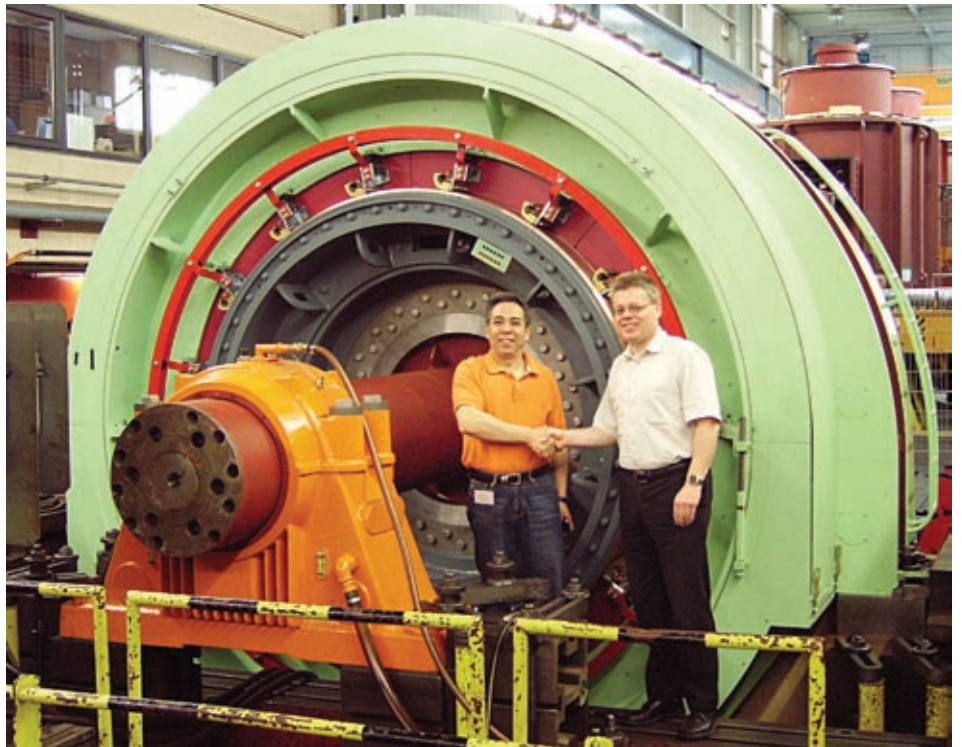
The new mining motor at LDW's test stand in Bremen. Guo Liang Huai (left), our representative in China, and Holger Rubach manage the project for LDW.
