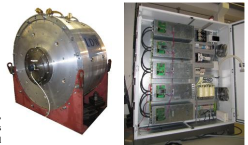
Fig. 11: The TFG and switchgear cabinet
